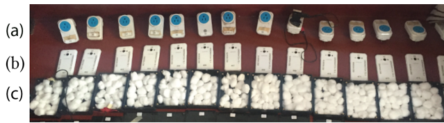
Figure 2: Plug load monitors and Android gateways before deployment. (a) The WiTenergy plug-load meters plug into an available wall outlet. (b) A phone plugs into the WiTenergy meter via a standard 5V DC USB adapter. (c) The cord from the adapter runs into a plastic box, which is padded with cotton balls and screwed shut. The phone sits in the box and runs the gateway application, forwarding data continuously from the WiTenergy to the cloud.
